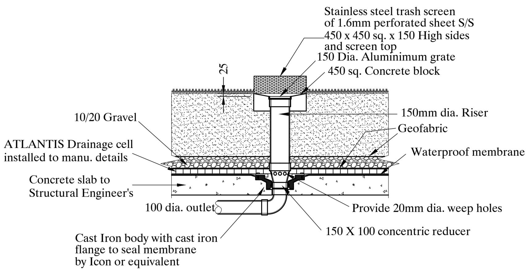
**TYPICAL LAWN INLET DETAILS ON SUSPENDED SLAB**
