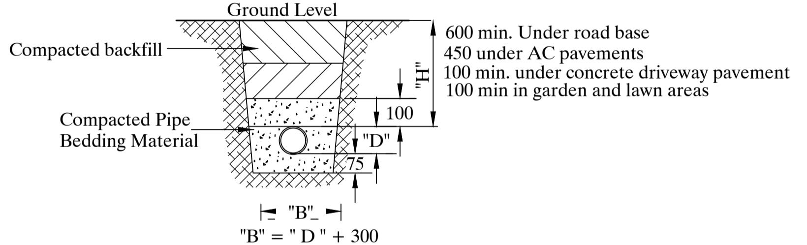
**TYPICAL SECTION OF P.V.C. UNDER GROUND STORMWATER DRAINAGE**
