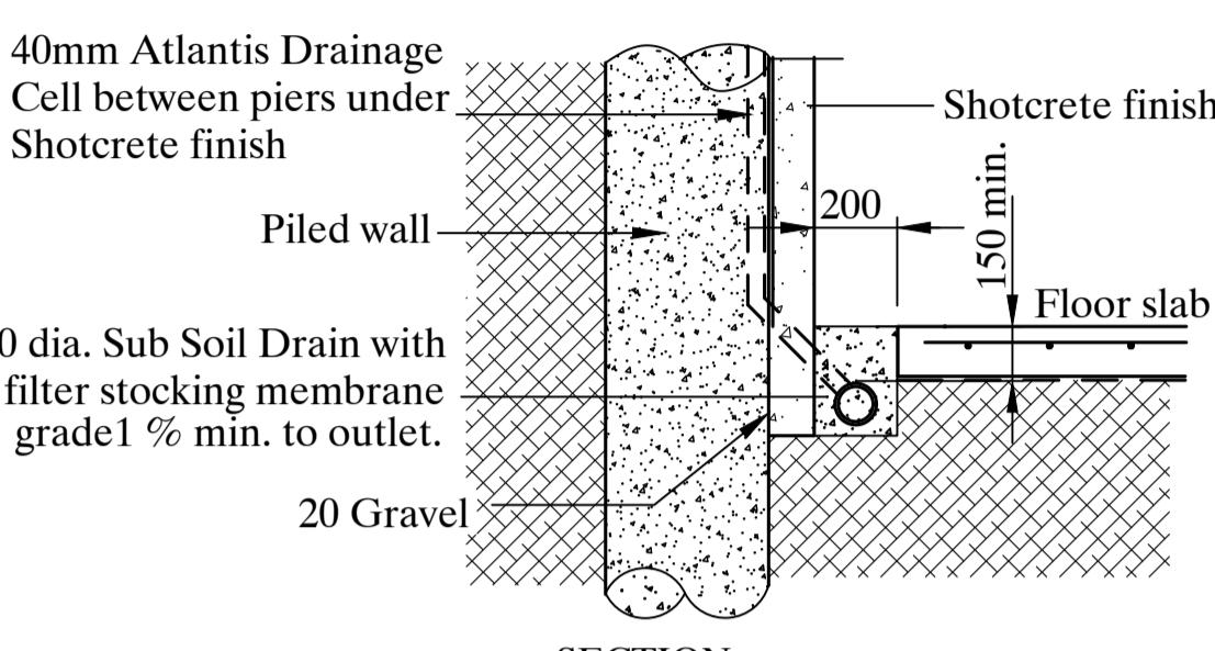
**TYPICAL SECTION SUB-SOIL DRAIN TO PILED BASEMENT WALL**
